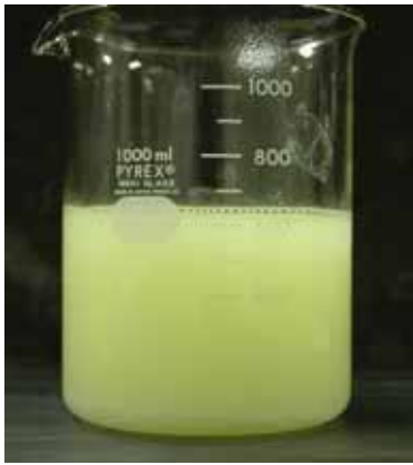
Fig.7 Representative photograph of emulsified gas oil (Water: 9 vol.% for Fuel, 800 rpm).
