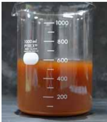
Fig.9 Representative photograph of emulsified A-Heavy oil (Water: 6 vol.% for Fuel, 800 rpm).
