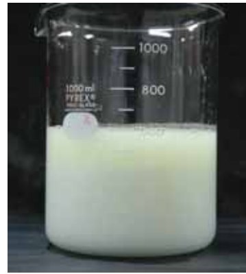
Fig.10 Representative photograph of O/W type emulsified gas oil due to the phase inversion from W/O type.
